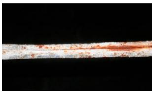
Coating: Heavy galvanized 230g/m<sup>2</sup> Wire diameter: 2,44 mm
