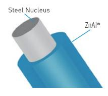
Complies with EN 10244-2. 'Steel wire & steel wire products. No ferric metallic recovering over steel wire. Part 2: Zinc recovering or Zinc alloy".
