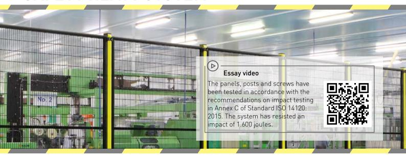
Framed panel in powder coated heavy steel wire allowing for different configurations (can be adapted for any length). The system also makes quick and efficient installation possible.
