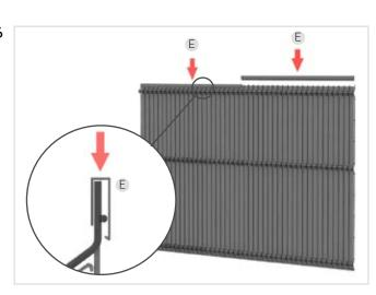
Did you know that you can also install the ReWood kit by braiding the vertical slats? You have the choice to do it with or without the V slats. It's a matter of aesthetics, the time it takes to install, but also a little trick to help hold the slats better on 1.20m high panels.
